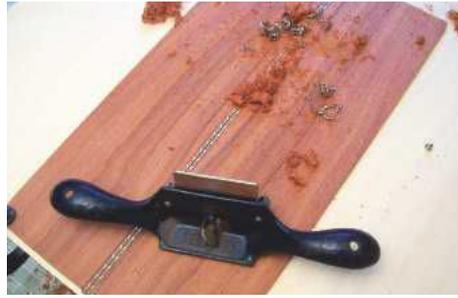
STEP 59. Thickening the back to 2mm with a scraper plane
