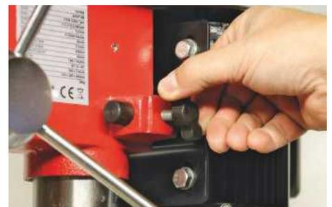
There are knobs on either side of the drill that tighten to these short stud bars...
