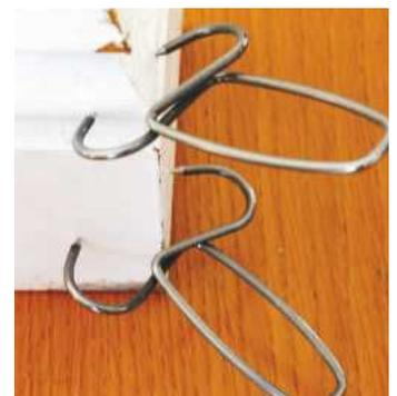
Spanning the joint to apply pressure to this skirting mitre
