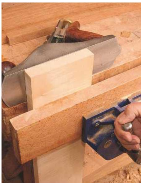
PIC 19. Ready for marking the dovetail sockets the wood is clamped in a vice with a plane used as a parallel-sided support alongside
