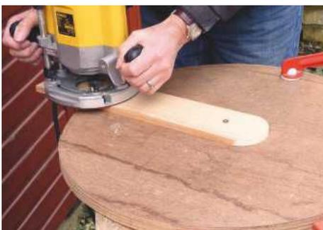
**STEP 10.** Screw the guide to the ply, then fit a sturdy straight cutter in the router and check the cut. Carefully rotate the router to clean up the edge
