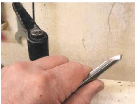
**STEP 5.** It's not only the tool you use that's important, it's also the way it's been sharpened. The 13mm signature gouge has been ground to a fingernail profile – as you'll see during the project, this will allow the use of push and pull cuts
