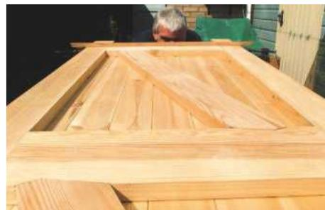
PIC 8. Checking for wind before clamping up
