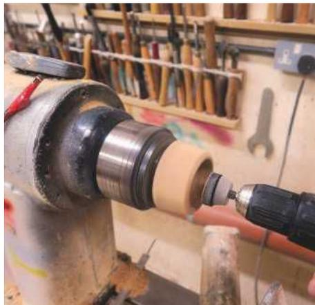
**STEP 23.** The easiest way to sand the flat inside of the lid is to use a 30mm sanding pad mounted in a drill. Be careful not to generate too much heat as the end-grain can crack
