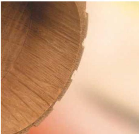
**STEP 22.** You should now have almost cut out to the correct diameter – here you can just see the remnants of the pencil mark. Remember to take small cuts: the lid does need to be tight so you can turn the top
