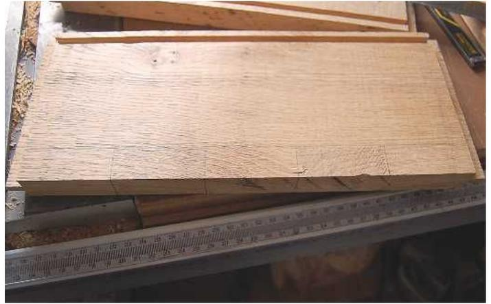
STEP 15. The hinge joints marked up
