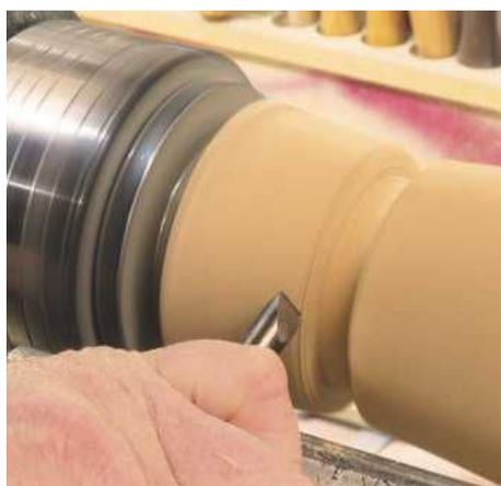
**STEP 14.** To chamfer or not to chamfer – that is the question! In the end I decided that it would look better if I cut an angle between the two mating parts of the box
