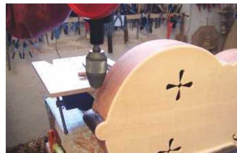
STEP 80. Drilling the tailblock to enable the tailpiece to be secured
