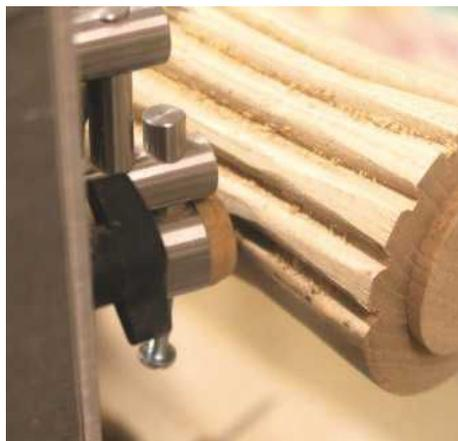
**STEP 11.** I found that working from right to left cuts cleaner than going the other way. The cutter has to be set on the centreline and ensure to watch out for the shavings building up in the depth stop
