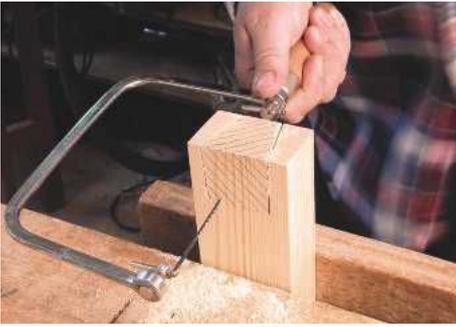
PIC 8. The sides or 'cheeks' of the socket are marked from the end down to the shoulder line, then waste is cut with a tenon saw and along the base using a coping saw
