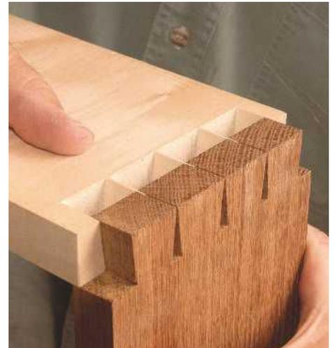
PIC 24. The fine dovetail joint is slid together
