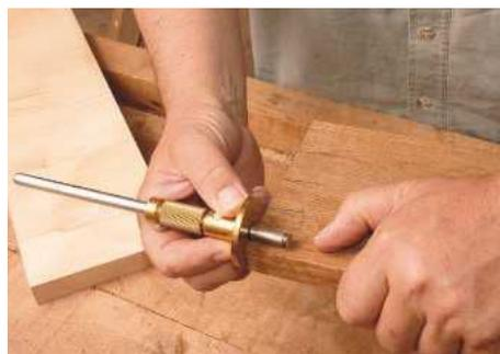
PIC 13. Keeping the marking gauge at the same setting, it is used to mark the shoulder line between the tails
