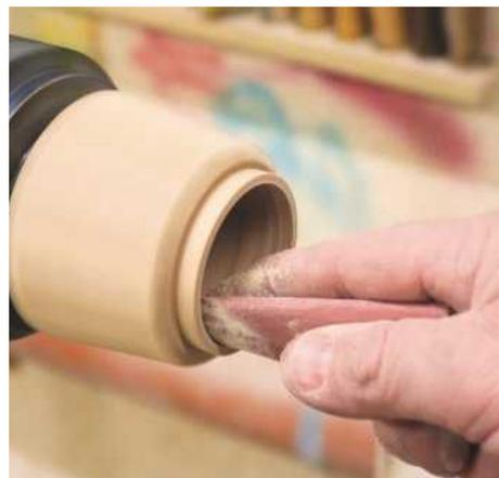
**STEP 30.** Start by sanding the inside of the box at 180 and work through to 400 grit. When sanding through a small hole like this, only place one finger inside, so nothing gets trapped
