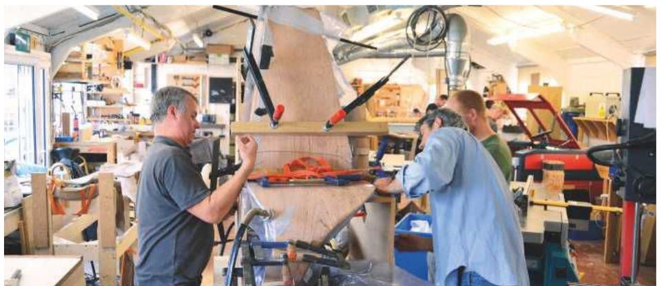
Vacuum bag, former and clamps required to hold the shape
