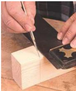
**PIC 3.** The shoulder lines run around the joint. By placing the knife blade in the previous line and sliding the square up against it, all four lines will join up accurately around the wood
