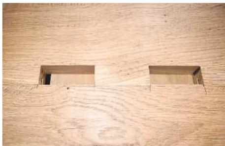
STEP 20. Using the joints on the back to mark the joint for the top
