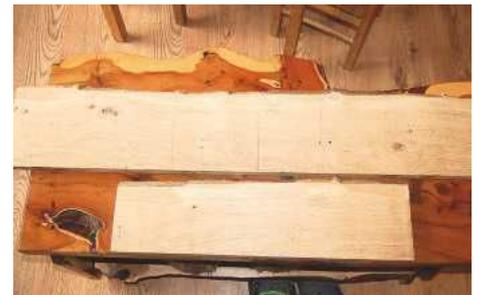
STEP 4. The parts of the jewellery box marked up, from top left to bottom right: lid, side panel, front, side panel and rear panel
