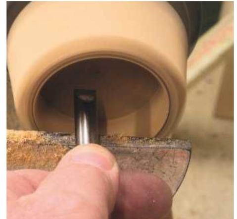
**STEP 21.** The same tool is used for creating a flat on the inside of the lid. Placing your finger on the toolrest will guide the depth of the tool as it's worked along the toolrest. Make sure the tool is presented on the centreline
