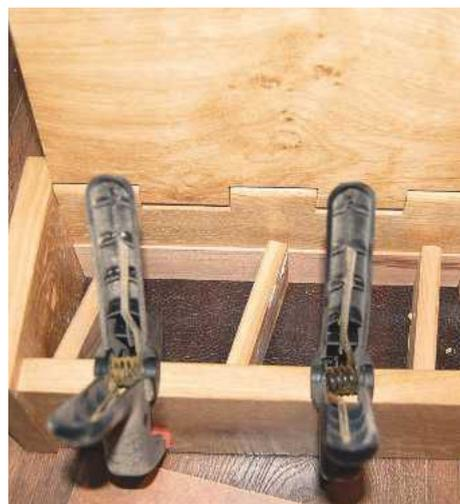
STEP 44. The box, with the trays in place, clamped up
