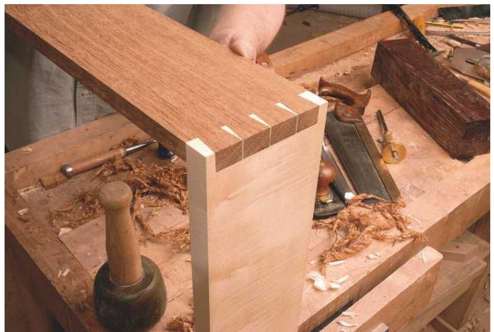
PIC 26. The outside of the finished joint shows the fine pins emphasised by the contrasting wood colours
