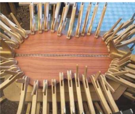
STEP 66. The back clamped into place
