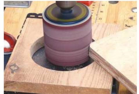
**STEP 3.** Cut each corner carefully with a jigsaw fitted with a narrow blade. Clean up these curves with a sanding drum or similar
