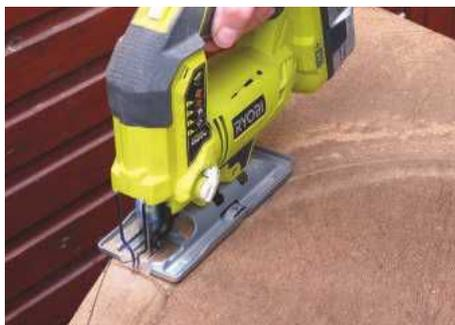
**STEP 8.** For a circular trolley, first draw the required radius using string and pencil. Cut the ply on the waste side of the line with a jigsaw
