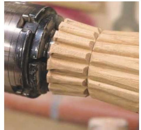
**STEP 24.** The base should fit perfectly onto the lid with a really tight fit and the diameters of the two sections should come together really well. At this stage, sand the box to a finish
