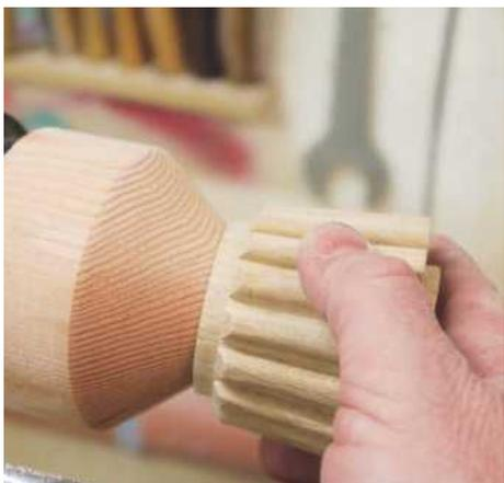
**STEP 31.** For this step you will need to turn yourself a jam chuck. Mount up a piece of softwood and turn a taper on the end; the box can then be offered up to give you an indication as to the correct diameter required between it and the wood
