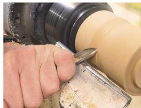
**STEP 6.** 'Push cut and bevel rubbing' is my preferred method for shaping effectively. The tool is cutting the fibres of the wood cleanly rather than scraping or breaking the wood away
