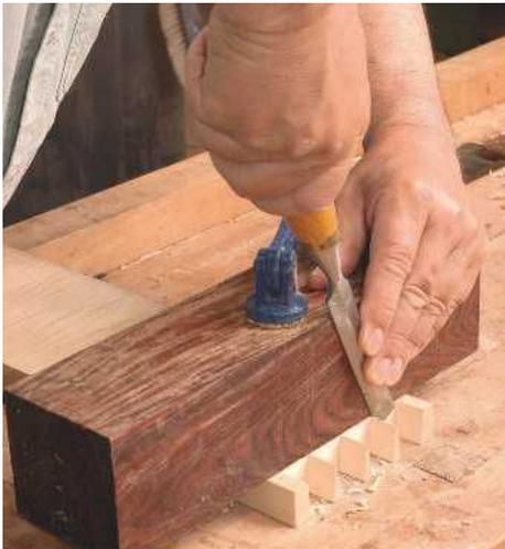
PIC 22. Socket bases are pared flat with a wide chisel using a block to guide the flat chisel back
