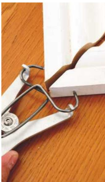
Applying a clamp to a mitre will bring it together tightly...
