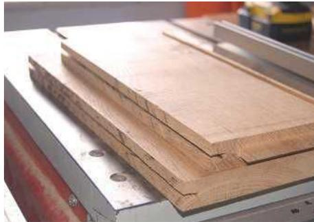
STEP 17. Slot cut to accept brass rod for the hinge
