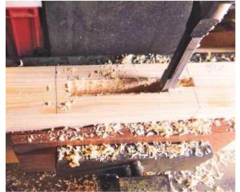
PIC 6. Cutting 15mm mortises with a 10mm chisel
