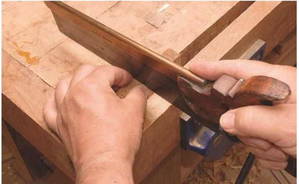
PIC 15. When starting a saw cut across the board the finger and thumb of the other hand are used to guide the position of the blade on the knife line
