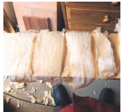
PIC 5. Nice wide shavings with a thick Ray Iles plane iron fitted
