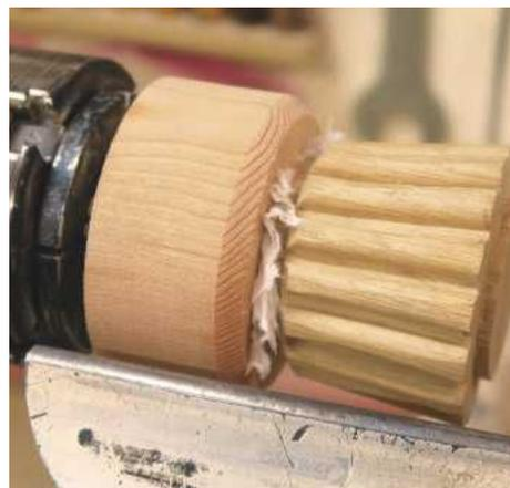
**STEP 33.** Whoops! I cut the jam chuck a little small so I had to use a piece of kitchen roll as a filler. Before you start turning, test the strength of the grip on the base
