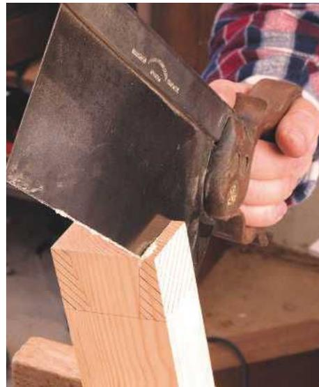
**PIC 5.** Shading pencil lines across the waste area helps keep track of which side of the line to saw against
