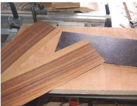
STEP 39. Leather on the inside and veneer for the bottom, which will cover the board
