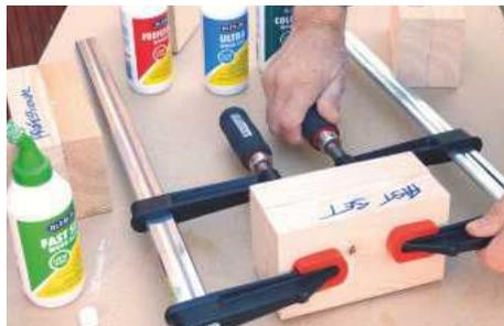
Using some freshly-planed softwood, I assembled several pieces as L-shaped corner joints, plus pairs of softwood blocks glued face to face
