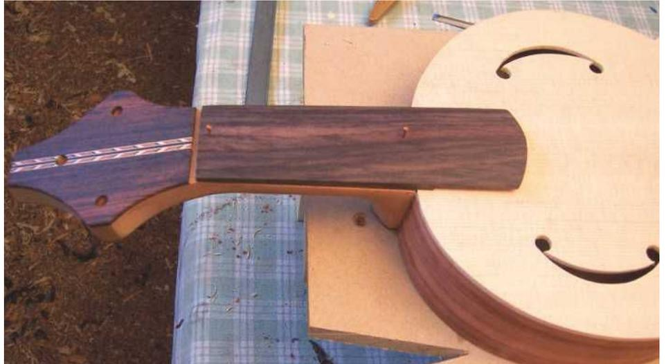
STEP 70. Pins are used to prevent the fingerboard from moving while the glue dries
