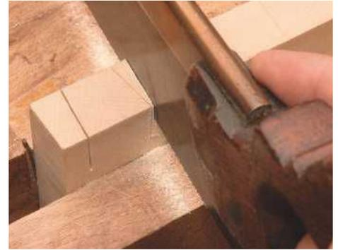
PIC 21. The pins are extremely narrow with the near side, little more than a saw-cut width
