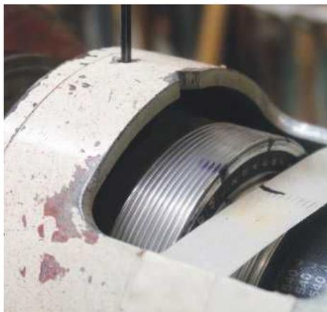
**STEP 10.** It's really important that the spindle is locked really tightly when routing as any sideways movement will give you wobbly lines. The box is going to be cut 16 times, so the indexing is 1, 4, 7, 10, etc. as it's a 48-point indexing wheel
