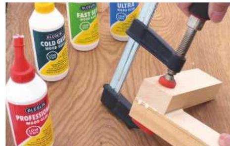
Each pair was cramped overnight with a heavy-duty F cramp, fully tightened
