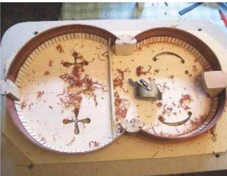
STEP 63. A thumb plane helps to level the ribs
