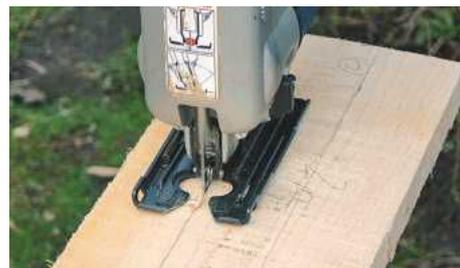
**STEP 2.** Although a table saw is faster and cuts straighter, its kerf is quite wide. A jigsaw, with a sharp blade, does the job almost as well with less waste
