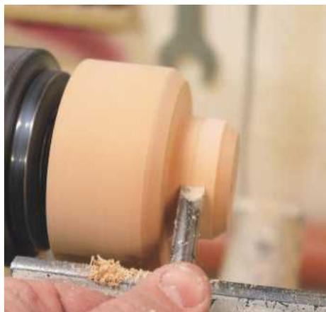
**STEP 32.** Use the 10mm skew to cut the timber down; this needs to be a tight fit into the base and the top of the box needs to come up against the shoulder
