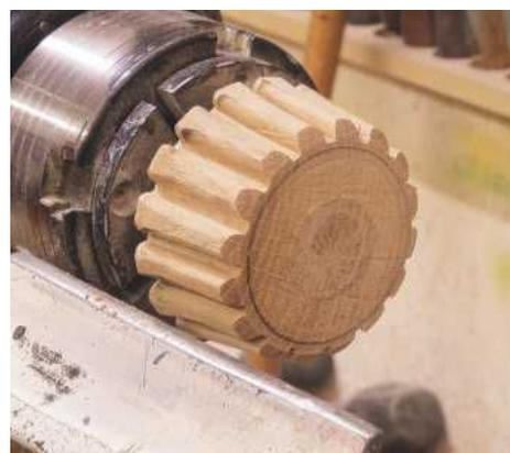
**STEP 18.** When you part it off ensure to leave a tiny amount of the spigot on the lid; this will be your guide for hollowing it out. The spigot should fit perfectly if you hollow to this line
