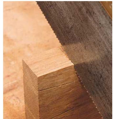
PIC 17. Sawing the end sockets with the blade cutting just inside the waste side of the shoulder line
