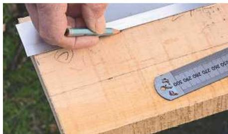
**STEP 1.** Select each hardwood board width for minimal waste. When marking out, allow about 5mm extra width on each piece for planing up
