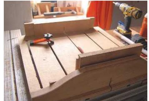
STEP 18. Cutting the hinges on my table saw using a cross-cut sled
