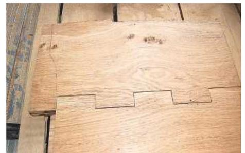
STEP 22. Testing the fit of the finger joints
