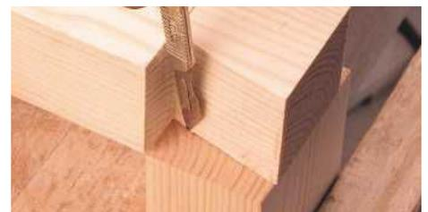
**PIC 7.** The dovetail is used as a template while the socket is marked around it
