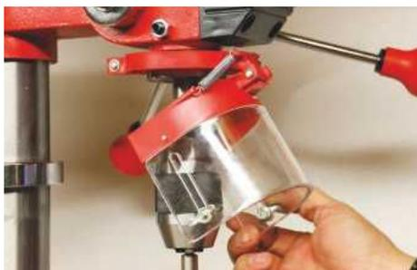
There's a flip up sprung safety guard supplied with the drill
