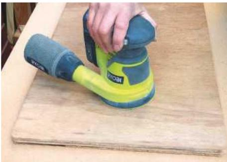
**STEP 4.** If necessary, sand the surfaces of each trolley with a random orbit sander, using 120 grit abrasive paper
