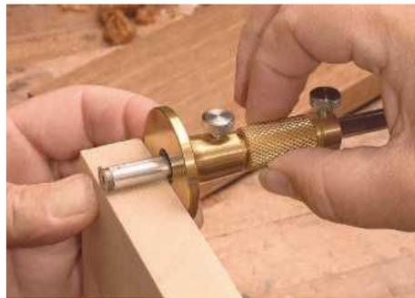
PIC 12. A marking gauge is set to the thickness of the wood that will carry the dovetail pins and sockets
