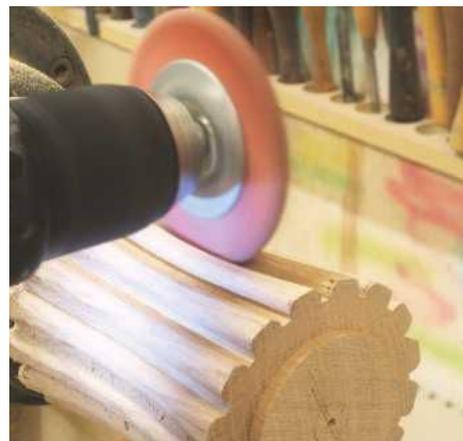
**STEP 12.** This nylon wheel just happens to be the correct width to fit in the grooves. Only do a rough sand at this stage as some more tooling will need to be added to the outside
