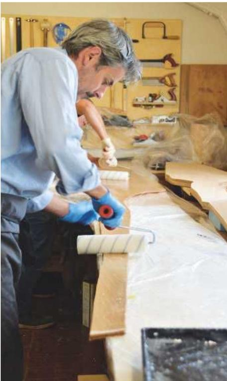
Using a roller to apply glues
