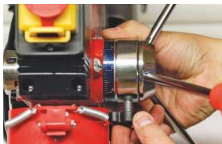
You can restrict the drilling depth with the knob and collar
