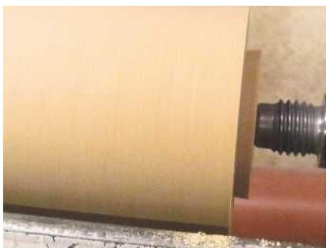
**STEP 4.** Next, a spigot needs to be cut on both ends. Making boxes does require a certain amount of accuracy and this spigot is perfectly cut, is the right diameter, with a small amount of dovetail to match the chuck jaws, and it's cut down cleanly so the top of the jaws will locate onto the blank
