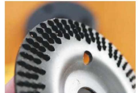
The R2 disc features a slight curvature, which will quickly shape profiles such as Windsor chair seats
