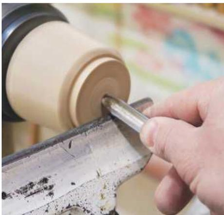
**STEP 28.** It's now time to hollow out the base, using the spindle gouge as before. I don't find there's a need to drill a depth hole and there should be no need to switch to a specialist hollowing tool until the overhang becomes over 75mm
