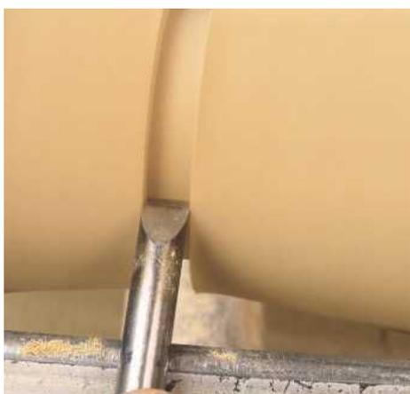
**STEP 13.** You can now begin to form the box by cutting the spigot for the base. Use a 10mm skew chisel to cut in 3mm below the bottom of the routed grooves; this will form the part which the lid fits over
