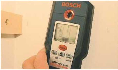
**STEP 6.** A detector for cables in the wall will prevent a potential accident when drilling. Sophisticated models detect timber studs, wires and metal pipes
