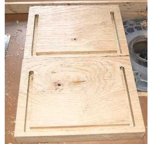
STEP 9. The dados on the two side pieces are longer towards the rear. More start and finish marks are added to the long piece on the right
