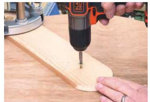
**STEP 9.** Make a routing guide from thin softwood or MDF. Bolt this to the router baseplate, then measure back the correct radius to find the centre of the circle
