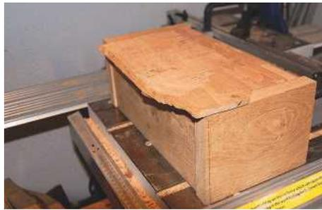
STEP 35. Checking the fit of the lid
