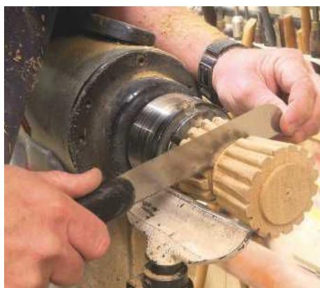
**STEP 17.** I would normally part all the way through and grab the bit as it comes off, but as it isn't too easy to hold due to its uneven surface, I decided to stop the lathe and cut the last bit through with a fine-tooth saw
