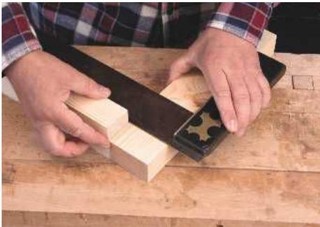
**PIC 2.** The position of the square used to mark the shoulder line is set from the thickness of wood on the other side
