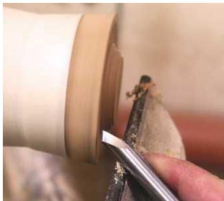
**STEP 26.** The position of the bevel is important when removing the spigot. The angle of the tool has to match the direction of the cut: if you present the tip of the tool to the surface, it will skate back
