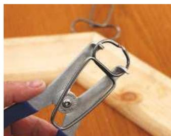
The clamps sit onto the pliers over the hooked ends
