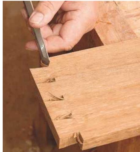
PIC 23. The inside corners of the tails are pared away to help the joint fit without jamming
