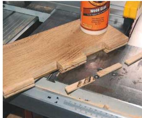
STEP 25. Inserting pieces cut to size ready to glue in the brass rod
