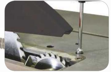
Height and side adjustment of the pre-scoring attachment. (Tool supplied). Precisa 6.0 VR -P1 only. Cannot be retro fitted.
