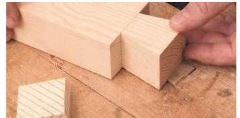
**PIC 6.** With waste cut off each side the single large dovetail is left
