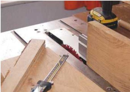
STEP 16. Doing a test cut on an offcut
