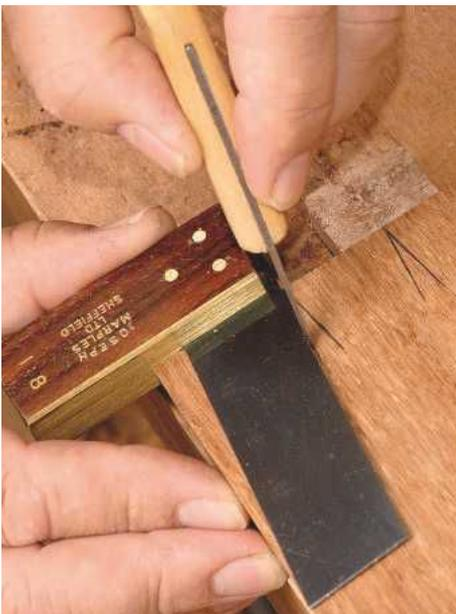
PIC 11. Dovetails marked across the width of a board are made so fine that the gaps between them will be no more than the width of a saw-cut or 'kerf'
