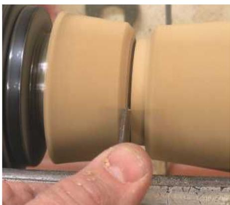
**STEP 16.** Part the base off using a 2mm parting tool – using such a thin tool ensures you don't waste too much timber. Be sure to check that the tool goes in square
