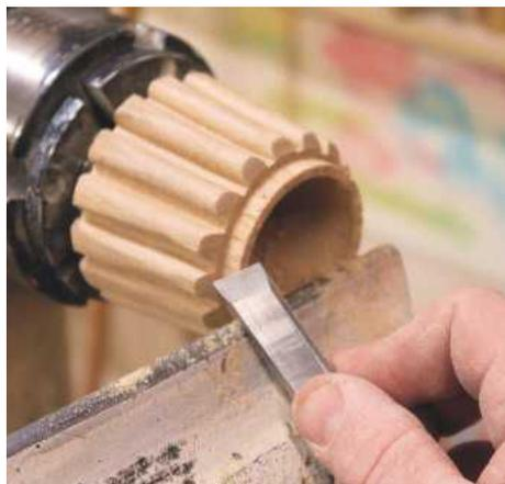
**STEP 29.** Due to the angle on the base, it's advisable to undercut the inside. My rolled edge skew has a 15° angle on the end and that matches the shape perfectly. I also sand the spigot so the lid will fit snugly and isn't over-tight
