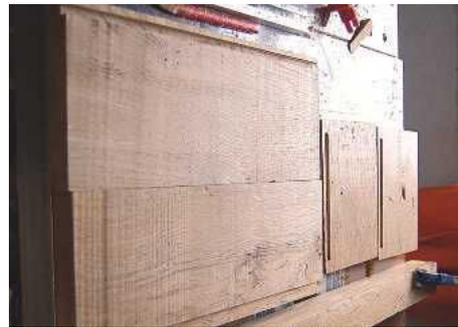
STEP 8. The piece on the left shows the full length of the front and rear panels
