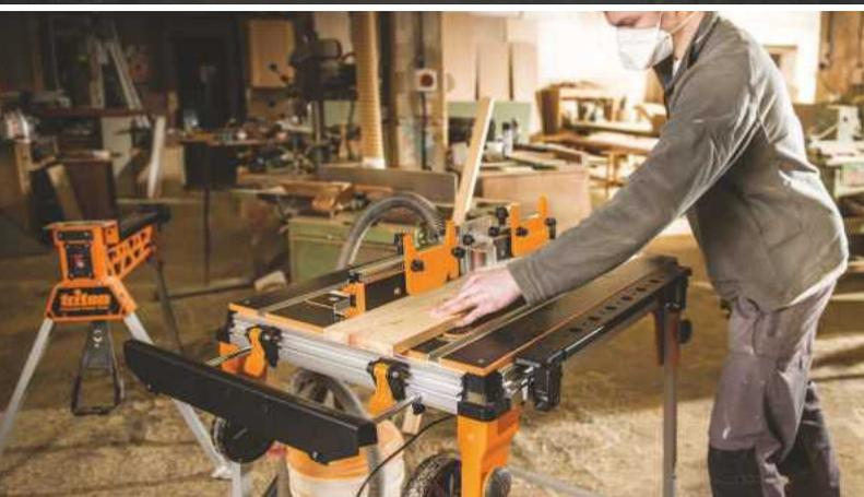
**Router Table Module** Precision router table & fence with featherboards
