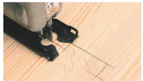
**STEP 17.** The most efficient way to saw pine, MDF or plywood shelves, is with a jigsaw. With a sharp blade fitted you can nibble edges to fit
