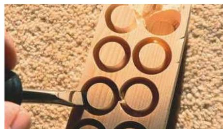
**STEP 5.** Use a plug cutter to make plugs from the same timber as the battens. To help match the grain, draw a pencil line along each row prior to removal
