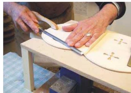
STEP 53. The harmonic bar is trimmed to length with a paring chisel
