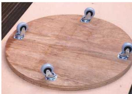
**STEP 11.** Fit at least four castors to the underside of the ply. Depending on loading, you may want to add another in the centre
