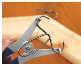
Squeezing the pliers opens the spring clamps very easily
