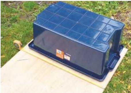
**STEP 1.** Measure the storage trunk or toolbox and mark out plywood or MDF for each trolley. Cut this to size with a circular saw
