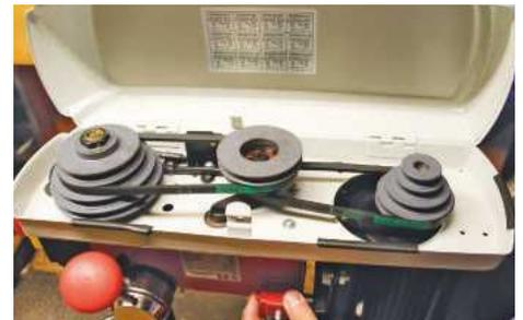
Finger pressure is enough to slide the motor back to re-tension
