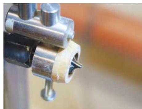
**STEP 9.** The cutting depth is determined by the wooden insert on the adjustable depth stop. This particular cutter has a flat end, which will create a cog effect more than one which goes to a point
