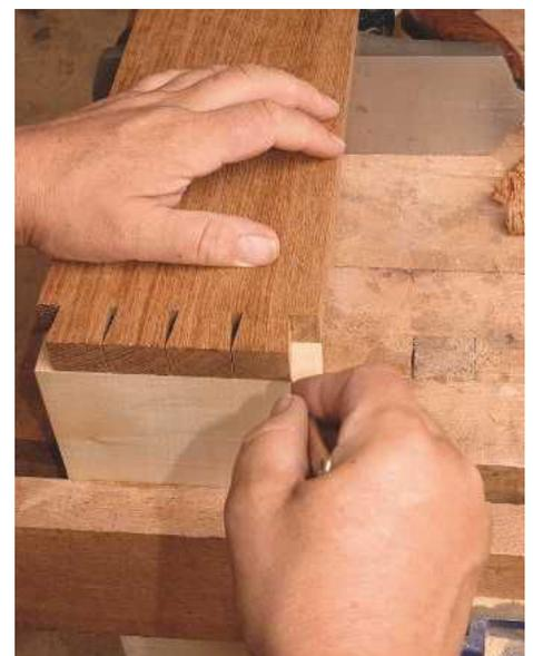
PIC 20. The dovetails are used as a template for marking out the sockets with a fine knife
