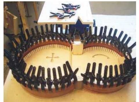
STEP 65. The completed linings in place ready to support the back
