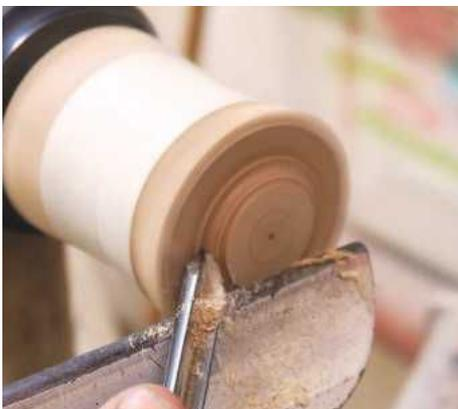
**STEP 25.** The base is mounted into the chuck and the lid is fitted on so the top can be turned. The masking tape is added for security; you could use the tailstock but I find it can get in the way
