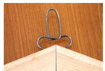
The design of the Spring Clamps allows them to span any mitre angle
