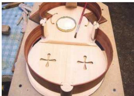
STEP 54. The rib blocks being glued into place
