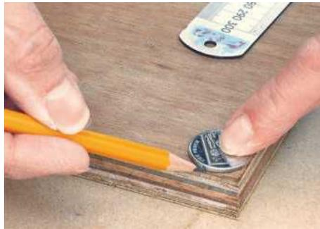
**STEP 2.** Clean up the edges and draw a suitable radius at each corner. Using a large coin is a quick way to do this
