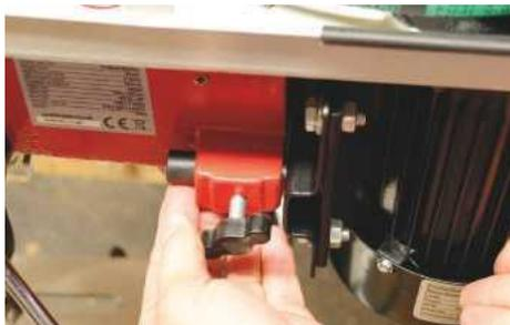
... which allow the motor to slide along the bars...
