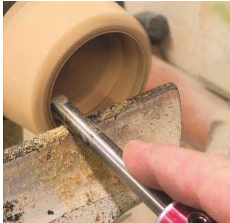
**STEP 20.** Once you have cut the majority of the wood out with the gouge, use the 10mm skew to true up the sides. Line the tool up with the bed of the lathe and push the tool straight into the end-grain
