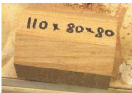
**STEP 1.** As we're going to stain the piece black, I recommend using European oak, which you need to make sure is free of splits and knots. Take the corners off to make roughing out quicker
