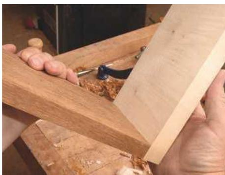
PIC 25. As the shoulder lines have been carefully aligned there are no gaps visible inside the joint
