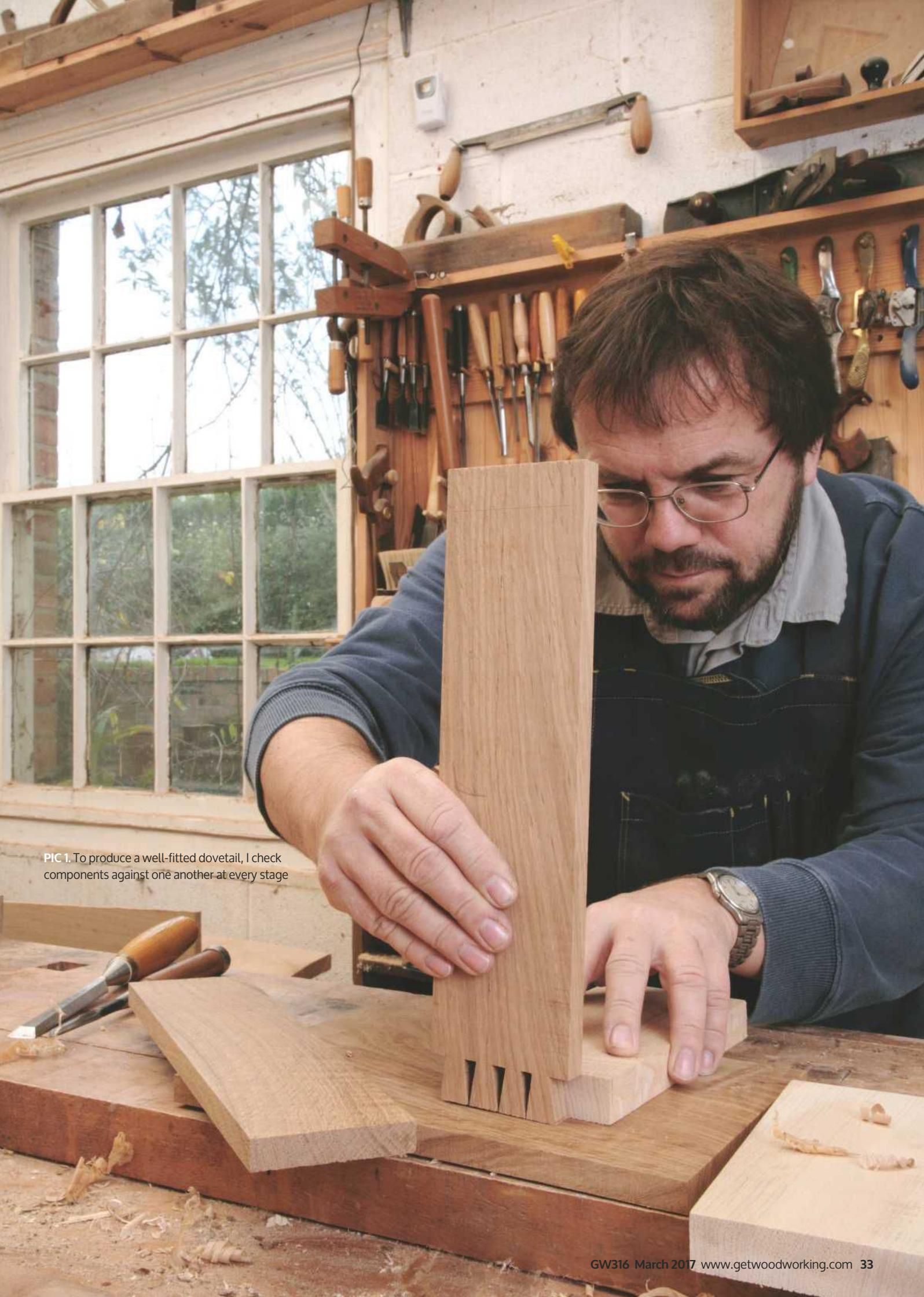
PIC 1. To produce a well-fitted dovetail, I check components against one another at every stage
