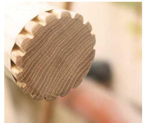
**STEP 27.** Chamfer the top of the box to match the join. Make sure you cut a slight concave into the base, which will allow the box to sit on its outer diameter, so it won't wobble
