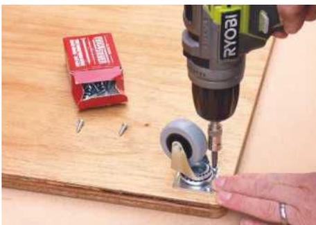
**STEP 7.** Mark the position of each castor on the underside of the trolley. Drill and screw the mounting plates to the plywood
