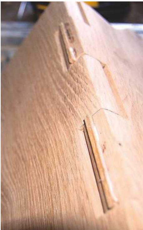
STEP 37. Lid fitted to the back and the final insert pieces added to complete the hinge mechanism
