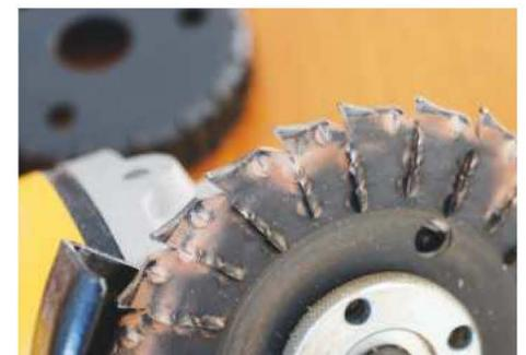
After a long run of work it still cuts quickly and cleanly with just a light build-up of dust
