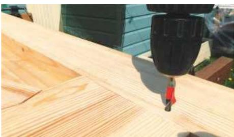
PIC 10. Drilling 6mm holes for the dowels
