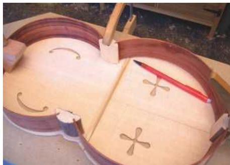
STEP 52. Marking the position of the ends of the harmonic bar
