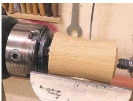
**STEP 7.** Take the diameter of the middle down by around 5mm to create a waisted shape that will add a little interest to the final box. The lid end should be held in the chuck
