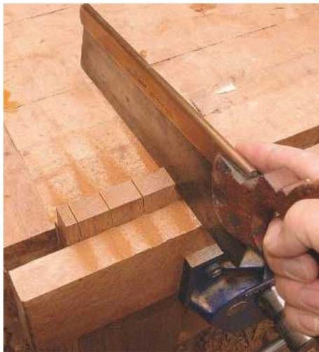
PIC 16. Using a small tenon saw or dovetail saw, the sockets between the tails are cut down as far as the shoulder line
