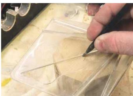
**STEP 2.** Mark the centres so it can be accurately mounted on the lathe. One of these plastic gauges is perfectly good for this. If the wood isn't entirely square, you will need to mark four times and take the average in the middle
