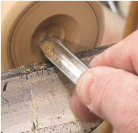
**STEP 19.** The 13mm signature gouge is now used in pull cutting mode. Make sure the flute is not pointing upwards: have it facing towards you, present the tool to the centre and then pivot it towards you, thus creating a dish
