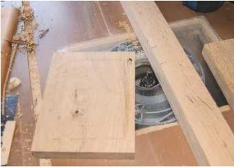
STEP 6. Here you can see the dado for the bottom of the box and the start and finish marks on the long piece of oak
