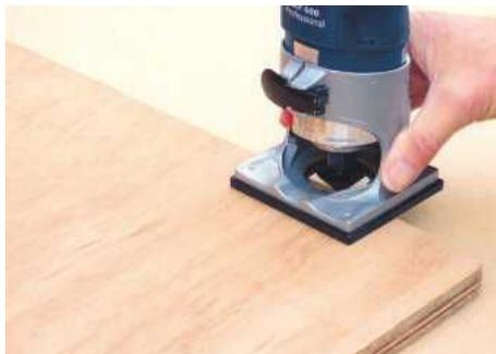
**STEP 5.** Rout a small chamfer around both upper and lower edges; this reduces the plywood splintering and improves handling
