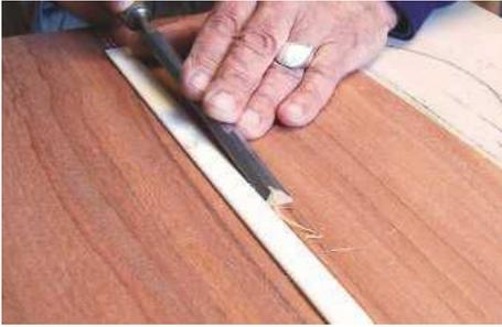
STEP 61. Removing glue squeeze-out with the aid of a paring chisel
