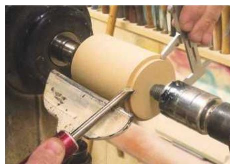
**STEP 3.** Make the work round with the spindle roughing gouge and use the 10mm skew chisel to cut the spigot. It's well worth practising to use this tool one-handed, so you can make this cut more easily
