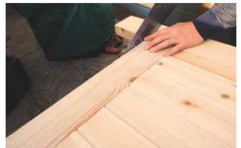
PIC 9. Cutting the horns after gluing up
